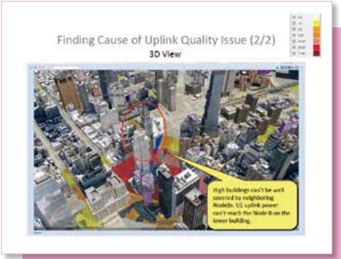
》 CovMo—Finding Cause of Uplink Quality Issue (3D View)
