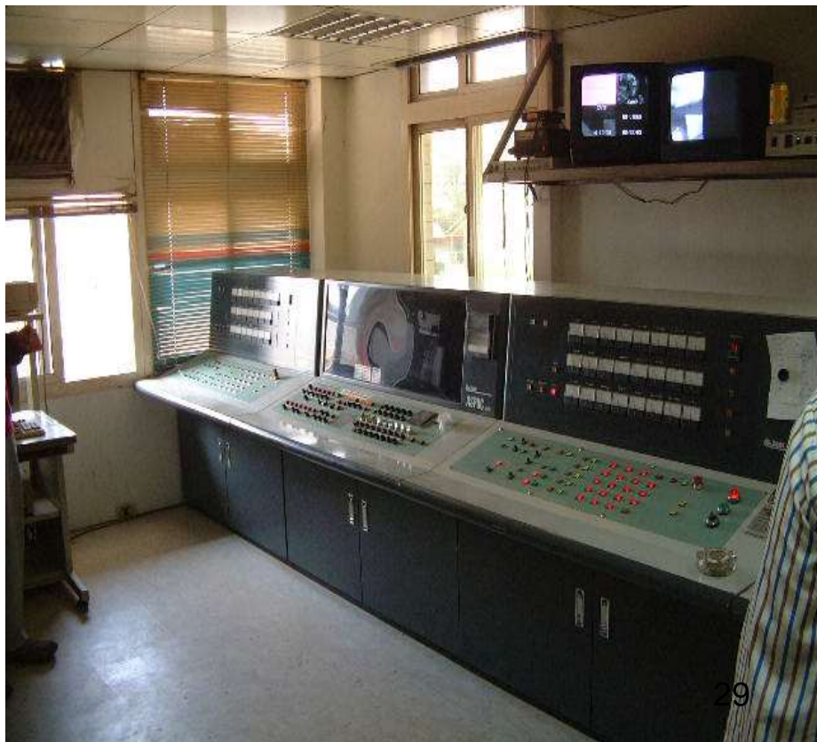
Photograph 12.8 – A modern drum mix plant control room (Photograph reproduced by kind permission of Redland Aggregates Limited)
