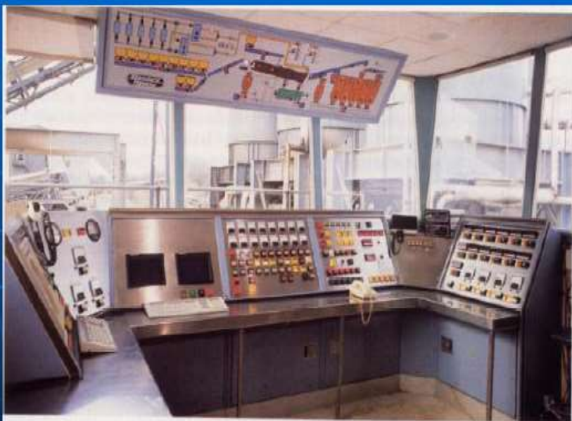
Photograph 12.8 – A modern drum mix plant control room (Photograph reproduced by kind permission of Redland Aggregates Limited)
